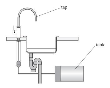
The system consists of a small tank connected to the water supply. Water in the tank is heated under pressure to a temperature of 110°C.
