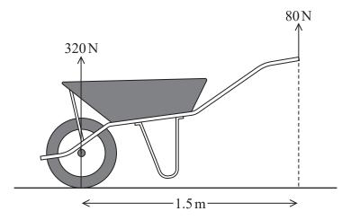
Determine the horizontal distance between the centre of gravity of the wheelbarrow and the centre of the wheel.
