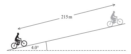
As the cyclist pedals, there is a constant forward force on the bicycle of 150 N. The cyclist travels 215 m along the slope.
