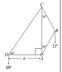
Draw a stress diagram using Bow's notation and **hence**, find the stresses in the rods stating whether they are tensions or thrusts.
